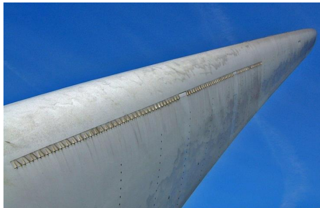
Wind turbine blade equipped with VG's (not the VORTEX GENERATOR PRO type of this brochure)
